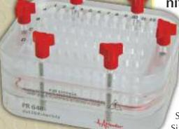
The PR648 supports screening as many as 48 samples quickly and easily without cross contamination between samples.
